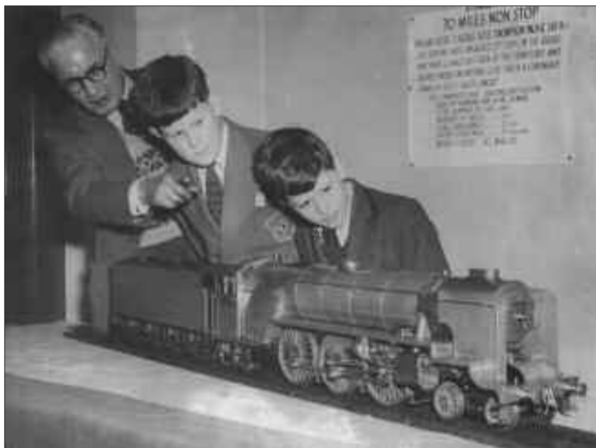
Two schoolboys admire the model of 'Hielan Lassie' an A2/3 Thompson Pacific at the 1955 Exhibition. The sign proclaims: 70 miles non stop. This run was made on August 21st 1954 on the Ridge Way Park (Chingford) track of the Chingford and District Model Engineering Club. This is a continuous track of 322.5 yards circuit. Trial commenced 10am. Trial concluded 8.10pm. Non stop running time 10 hrs 10 mins. Total number of laps 383. Number of miles 70. Coal consumed 25 lbs. Water consumed 23 gallons. Drivers E. Jater and A. E. Waller. Photo: MRC Collection.
